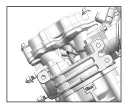
Measure the electrode gap with a thickness gauge, and if necessary, adjust the gap to specification.
