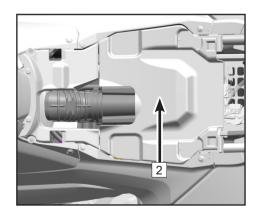
lubricant on the inside diameter of the air filter rubber seal.
